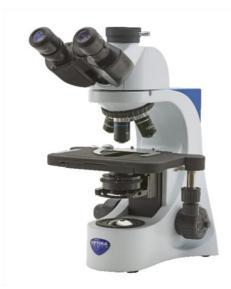
Trinocular brightfield microscope, 1000x, IOS N-PLAN objectives
